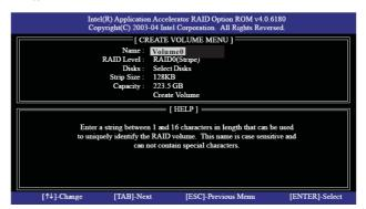
Use the up or down arrow keys to select your desired **RAID** Level. You may select RAID 0 (Stripe), RAID 1 (Mirror), RAID 5 or RAID 10 for your RAID level. Press <Enter>, and then you can select **Strip Size**.
