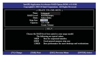
If you selected RAID 0 (Stripe), use the up or down keys to select the stripe size for your RAID 0 array then press <Enter>. The available values range from 8 KB to 128 KB. The default selection is 128 KB. The strip value should be chosen based on the planned drive usage.
